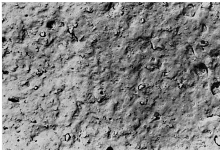
Fig. 12. Electron microscope photograph for the 16.8% volume HAF (heat-treated compound).
